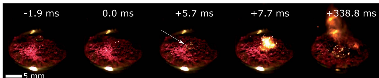
Fig. 3 Example of a ignition drop test on 50 wt% FR5560 wax/50 wt% \text{Co(AlIm)}_2 using WFNA as the oxidizer. The location of the first ignition is marked with the white arrow. Full sequence available on ESI.†
