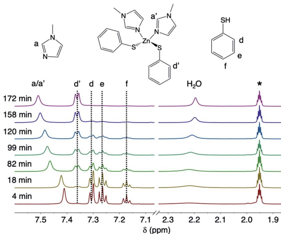
Fig. 2 Stacked room-temperature solution <sup>1</sup>H NMR spectra in acetonitrile-*d*<sub>3</sub> of the aromatic region and H<sub>2</sub>O peak for aliquots taken as a function of time from the dissolution of ZnO with MeIm and thiophenol at 75 °C. Acetonitrile-*d*<sub>2</sub> is labeled as \*. Full spectra are provided in the ESI.<sup>†</sup>
