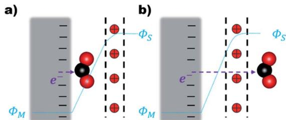
Fig. 1 (a) Inner-sphere and (b) outer-sphere electron transfer from the cathode to  $\text{CO}_2$ . The red positive charges within the black dotted lines denote the EDL. ( $\Phi_M$ ) and ( $\Phi_S$ ) are the surface and bulk solution phase potentials respectively.
