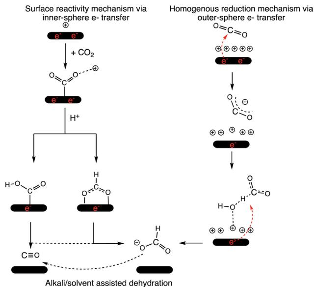
**Scheme 1** Mechanism of the CO<sub>2</sub>RR over a cathode surface *via* inner- and outer-sphere electron transfer. 2e<sup>-</sup> that originate from the cathode surface and reduce the CO<sub>2</sub> moiety are shown in red for representative purposes. The cathode surface is maintained at a constant potential in the electrolyzer.
