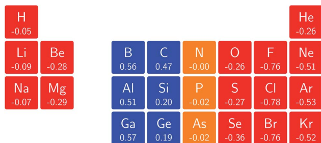
Fig. 8 Initial responses of the electronegativity in a magnetic field as a periodic table representation showing both the numerical values and categorising them with a color code in which blue indicates a positive derivative, red a negative derivative and yellow a derivative that is zero or close to zero.
