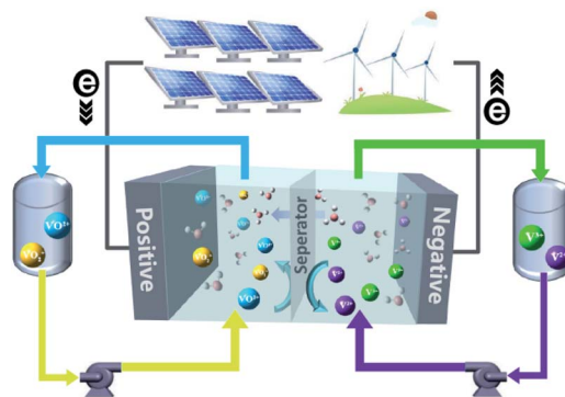
Fig. 1 A schematic diagram of a VFB.
