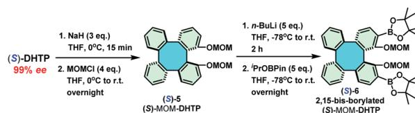
**Scheme 6** Synthetic routes for methoxymethylation and borylation of (*S*)-DHTP. MOM = methoxymethyl, Pin = pinacol, and <sup>1</sup>PrOBPin = 2-isopropoxy-4,4,5,5-tetramethyl-1,3,2-dioxaborolane.
