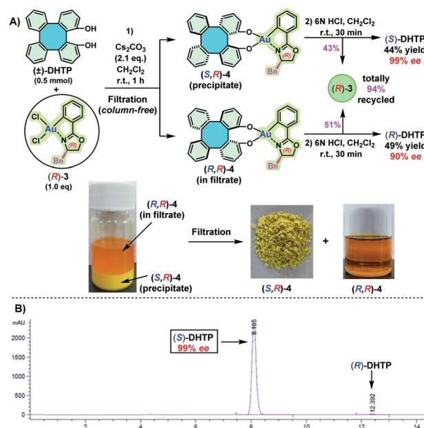
Scheme 3 (A) Optical resolution of ( $\pm$ )-**DHTP** by using enantiopure (*R*)-**3**. Reaction conditions: step (1): ( $\pm$ )-**DHTP** (0.5 mmol), (*R*)-**3** (0.5 mmol), Cs<sub>2</sub>CO<sub>3</sub> (2.1 eq.), CH<sub>2</sub>Cl<sub>2</sub> (10 mL), room temperature (25 °C), reaction time: 1 h; step (2): CH<sub>2</sub>Cl<sub>2</sub> (10 mL), HCl (6 N, aq.), room temperature, reaction time: 30 min. Yield of the isolated product. (B) HPLC spectrum of the obtained (*S*)-**DHTP**. Bn = benzyl.
