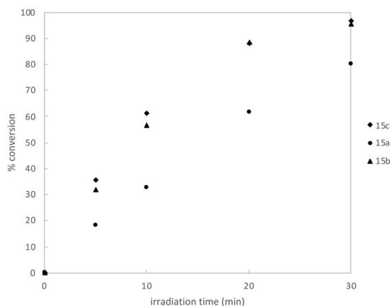
Fig. 2 Kinetic profile of irradiation of acyl silane probes in MeOH- $d_4$  ( $n = 3$ , average) using a 6 W handheld UV lamp at 365 nm. Conversion was determined by  $^1\text{H}$  NMR using an internal standard. Full details available in ESI.†
