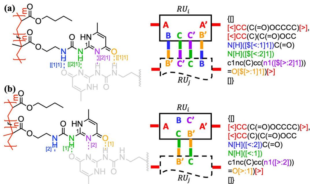
Fig. 6 The indexing of non-covalent BigSMILES to annotate poly(*n*-butyl acrylate-*co*-UPy) polymers representing (a) fully correlated and (b) independent connectivity patterns.<sup>52</sup> From left to right of each figure are the detailed chemical structures, the generic connectivity patterns between RUs, and their associated BigSMILES syntax respectively.
