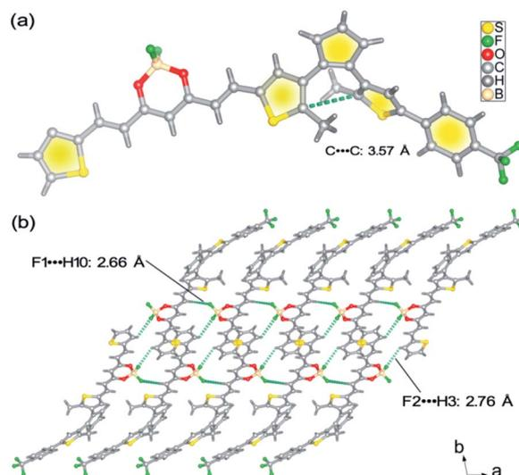
**Fig. 1** (a) Crystal structure of the **BFBFDTETe** molecule. (b) View of the 1D chain structure of **BFBFDTETe** extended by C–H $\cdots$ F hydrogen bonding.
