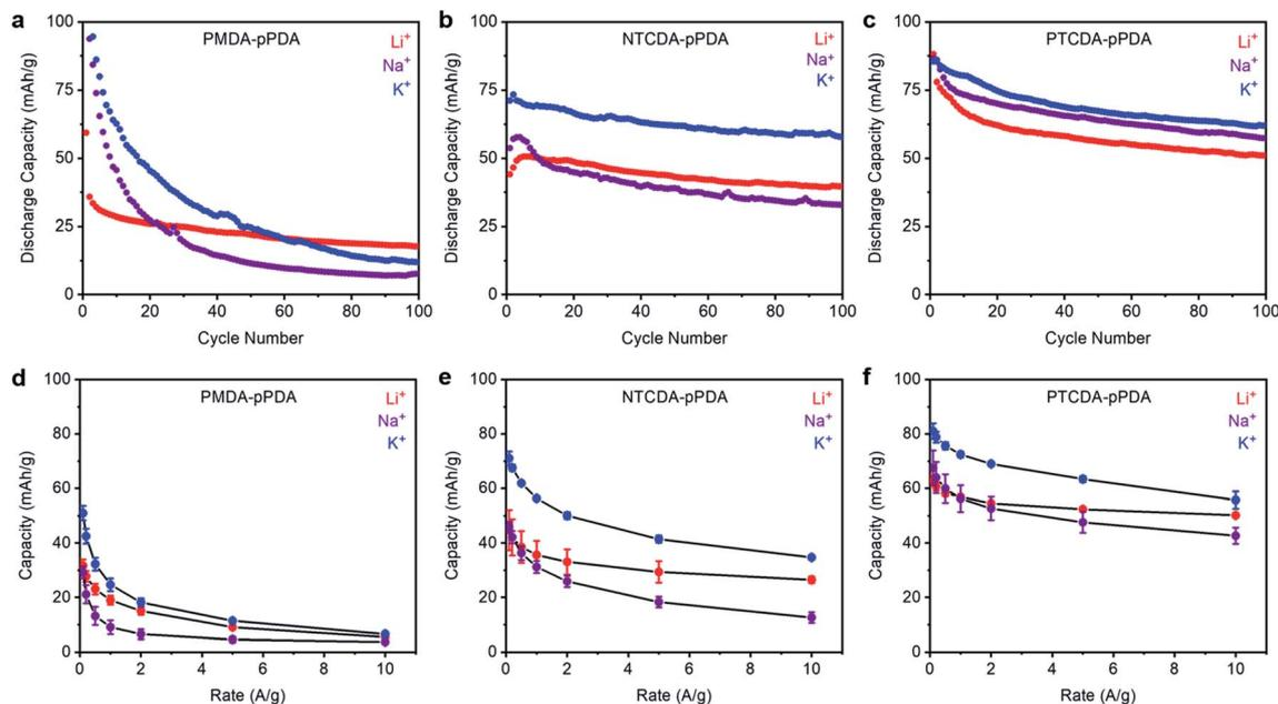
Fig. 3 Cycling performance of (a) PMDA-pPDA, (b) NTCDA-pPDA, and (c) PTCDA-pPDA in metal (Li, Na, K) half cells at a discharge rate of  $100 \text{ mA g}^{-1}$ . Average discharge capacities from rate tests for (d) PMDA-pPDA, (e) NTCDA-pPDA, and (f) PTCDA-pPDA in Li, Na, and K cells. The error bars represent one standard deviation of error in the measured capacity, determined from data obtained from at least three coin cells.
