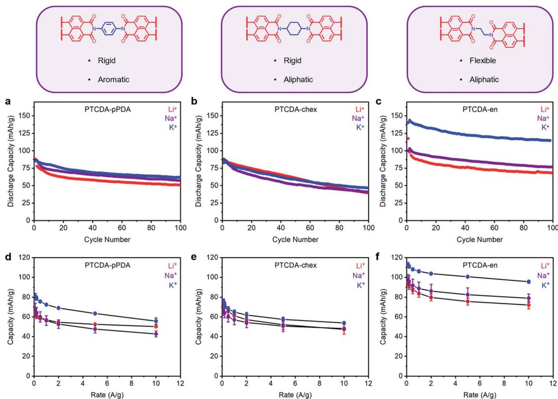
Fig. 4 Structural descriptions and cycling performance of (a) **PTCDA-pPDA**, (b) **PTCDA-chex**, and (c) **PTCDA-en** in metal (Li, Na, K) half cells at 100 mA g<sup>-1</sup>. Average discharge capacities from rate tests for (d) **PTCDA-pPDA**, (e) **PTCDA-chex**, and (f) **PTCDA-en** in Li, Na, and K cells. The error bars represent one standard deviation of error in the measured capacity, determined from data obtained from at least three coin cells.
