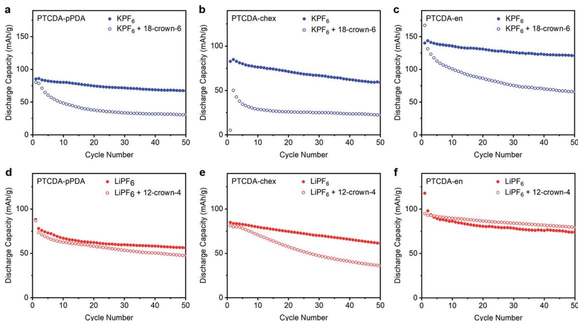
Fig. 5 Cycling performance at  $100 \text{ mA g}^{-1}$  for (a) **PTCDA-pPDA**, (b) **PTCDA-chex**, and (c) **PTCDA-en** in metal half cells containing  $0.8 \text{ M KPF}_6$  with and without  $0.8 \text{ M 18-crown-6}$  ether and (d) **PTCDA-pPDA**, (e) **PTCDA-chex**, and (f) **PTCDA-en** in cells containing  $1.0 \text{ M LiPF}_6$  with and without  $1.0 \text{ M 12-crown-4}$  ether.
