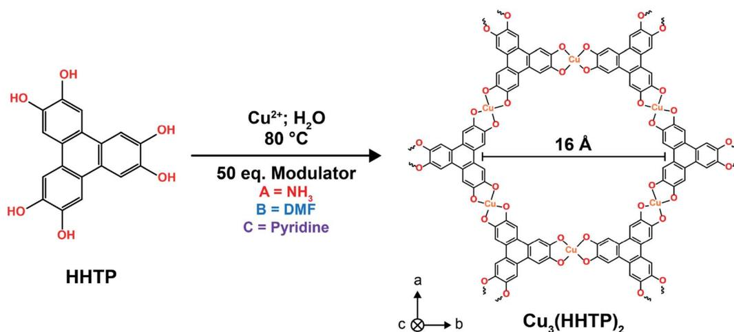
Fig. 1 Scheme for the hydrothermal synthesis of  $\text{Cu}_3(\text{HHTP})_2$  samples from 2,3,6,7,10,11-hexahydroxytriphenylene and a  $\text{Cu}(\text{II})$  precursor with different modulators. The structure of  $\text{Cu}_3(\text{HHTP})_2$  is shown on the left. This MOF is formed of  $\pi$ -d conjugated 2D sheets, which stack to form an extended 3D pore network.
