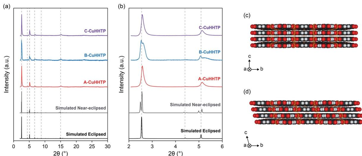
Fig. 2 (a) Experimental XRD patterns from A-CuHHTP, B-CuHHTP and C-CuHHTP compared to the simulated XRD patterns from  $\text{Cu}_3(\text{HHTP})_2$  with both eclipsed and near-eclipsed stacking sequences, and (b) zoomed view to show the differences in peak splitting between the three samples. (c) and (d) Structural models of  $\text{Cu}_3(\text{HHTP})_2$  with hexagonal eclipsed and monoclinic near-eclipsed crystal structures, respectively.
