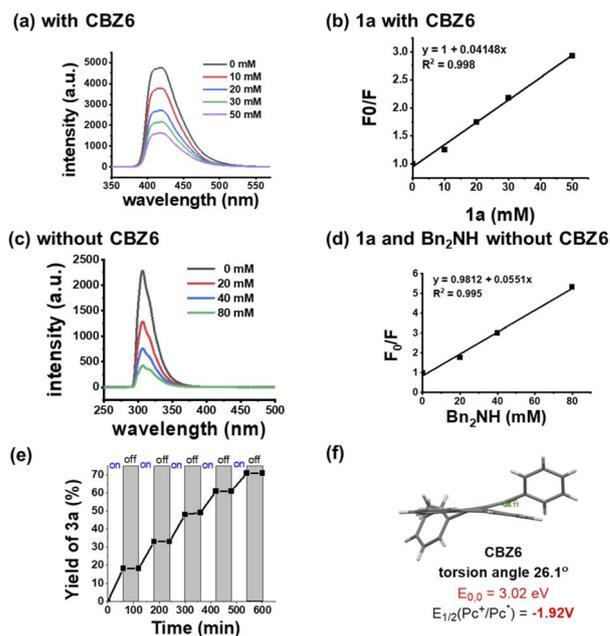
Fig. 6 Control experiments: the (a) fluorescence quenching effect between **1a** and CBZ6, (b) Stern–Volmer plot (**1a** vs. CBZ6), (c) fluorescence quenching effect between **1a** and **4a** (note: no effect above 400 nm), (d) Stern–Volmer plot (**1a** vs. **4a**), (e) on–off control, and (f) the molecular structure of CBZ6.
