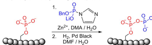
(b) Peptide pyrophosphorylation by using phosphorimidazolide and subsequent hydrogenolysis
