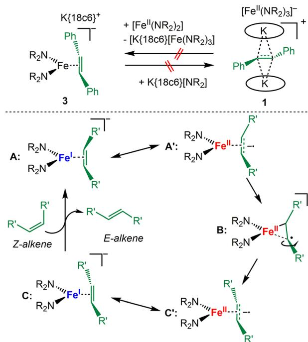
Scheme 4 Top: Attempted conversion of **3** and **1** into each other. Bottom: Proposed mechanism for the *Z* to *E* isomerization of alkenes with  $[\text{Fe}]$  as catalyst. Coordination of the *Z*-alkene to the metal ion as  $\pi$ - (A) or radical anion (A') complex; B: rotation along the C–C bond; C/C' *E*-alkene complex.
