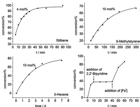
Fig. 4 Catalytic *Z* to *E* conversion for stilbene (top left),  $\beta$ -methylstyrene (top right), 3-hexene (bottom left) using  $[\text{Fe}^{\text{I}}]$  as catalyst and poisoning experiment with 2,2'-bipyridine (bottom right).
