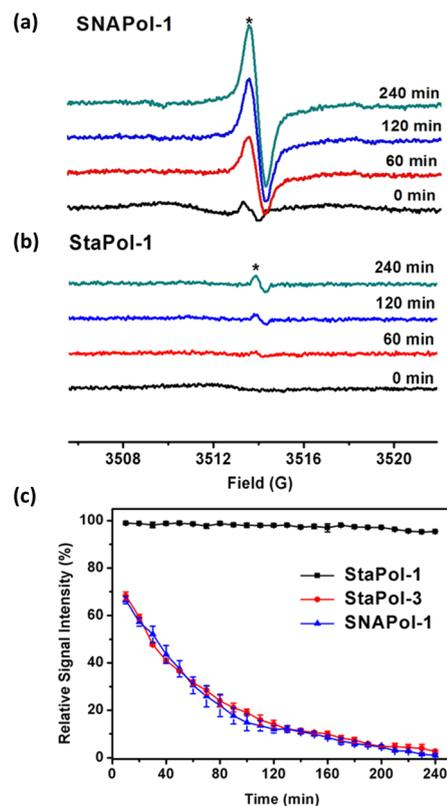
Fig. 3 EPR spectra of (a) SNAPol-1 (50  $\mu\text{M}$ ) or (b) StaPol-1 (50  $\mu\text{M}$ ) after incubation with cell lysates at different times (\*the signal from the trityl radical). (c) Time course of relative EPR signal intensity of biradicals (StaPol-1, StaPol-3 and SNAPol-1) after incubation with cell lysates.
