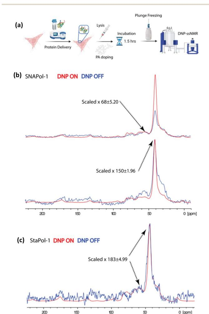
Fig. 6 (a) Scheme showing HeLa cell lysate preparation. (b and c) 1D  $^1\text{H}$ - $^{13}\text{C}$  cross polarization of HeLa cell lysates doped with 30 mM SNAPol-1 (b) or 30 mM StaPol-1 (c). Enhancement errors are calculated as detailed in the section of Materials and methods of the ESI.<sup>†</sup>
