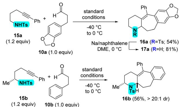
Scheme 5 Carbocyclization for synthesis of fused piperidines.
