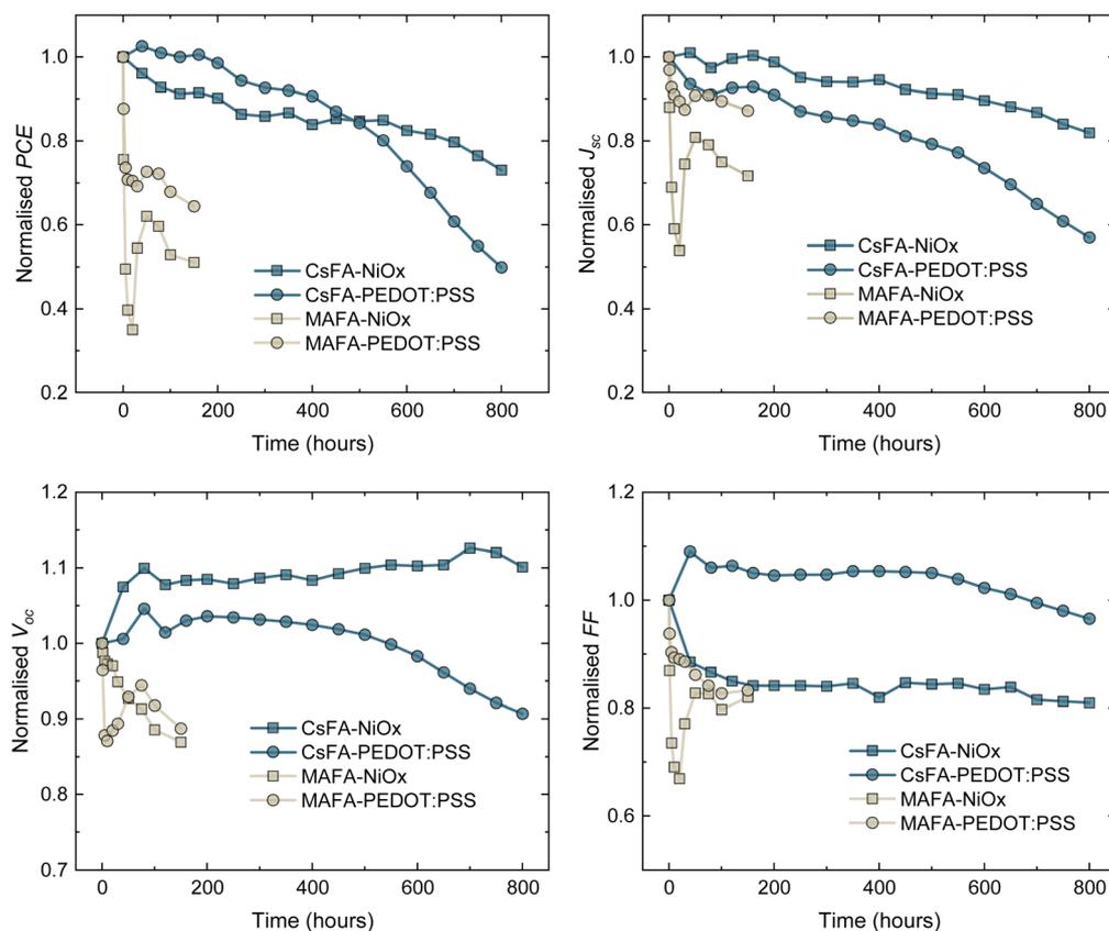
Fig. 4 Photovoltaic performance at 1 sun (metal halide lamp) as a function of time of unencapsulated MAFA and CsFA devices with  $\text{NiO}_x$  and PEDOT:PSS as the HTL.  $J$ - $V$ s were recorded each 10 min while devices were held at MPP under continuous  $\text{N}_2$  flow.
