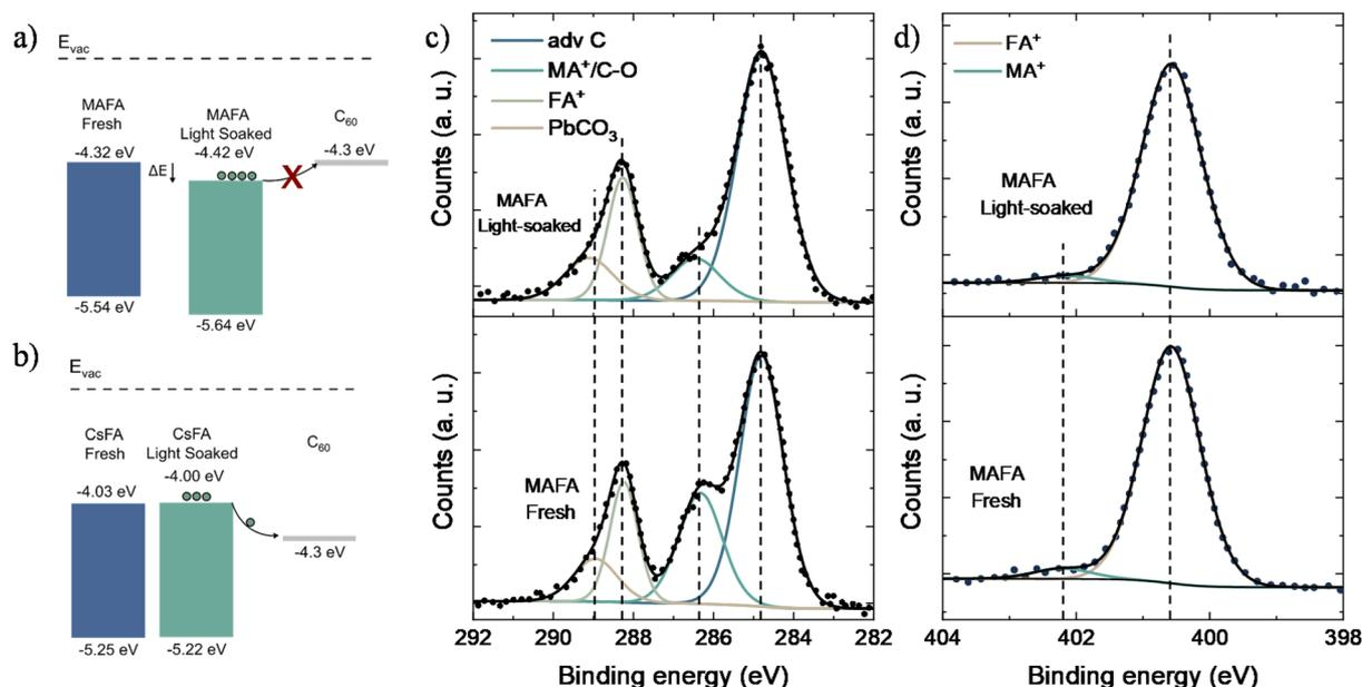
Fig. 3 (a) Band diagram of fresh and light soaked MAFA films highlighting the energy barrier between light soaked MAFA and  $C_{60}$ . (b) Band diagram of fresh and light soaked CsFA films. (c) XPS spectra showing the C 1s peaks of MAFA fresh and light soaked films for 6 h. (d) XPS spectra showing the N 1s peaks of MAFA fresh and light-soaked films for 6 h.
