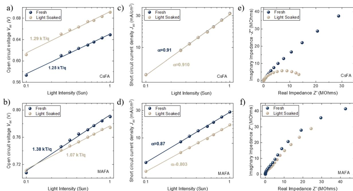
Fig. 2 (a and b) Light intensity-dependent  $V_{oc}$  measurements for CsFA and MAFA devices, (c and d) light intensity-dependent  $J_{sc}$  measurements for CsFA and MAFA devices, and (e and f) Nyquist plots derived from impedance spectroscopy measurements of CsFA and MAFA devices; measurements were taken in a N<sub>2</sub> atmosphere under dark conditions.
