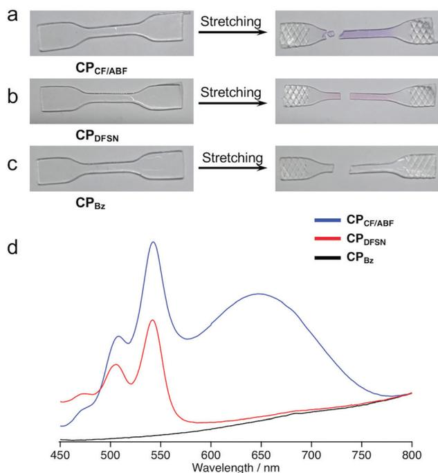
Fig. 4 Photographs of (a)  $\text{CP}_{\text{CF/ABF}}$ , (b)  $\text{CP}_{\text{DFSN}}$  and (c)  $\text{CP}_{\text{Bz}}$  films before and after fracture. (d) UV-Vis spectra of  $\text{CP}_{\text{CF/ABF}}$  (blue),  $\text{CP}_{\text{DFSN}}$  (red) and  $\text{CP}_{\text{Bz}}$  (black) films after fracture.
