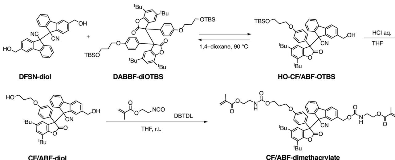
Scheme 1 Synthetic route to the CF/ABF cross-linker (**CF/ABF-dimethacrylate**).
