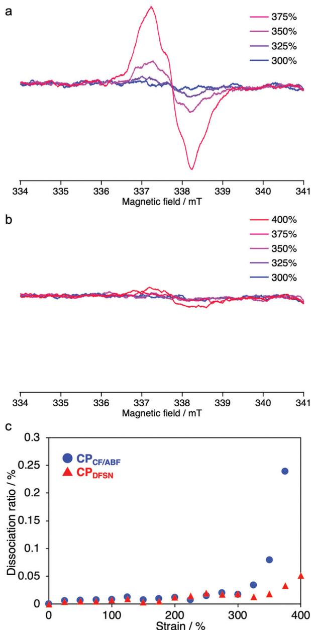
Fig. 6 EPR spectra of (a) CP<sub>CF/ABF</sub> and (b) CP<sub>Dfsn</sub> at each strain (100 mm min<sup>-1</sup>). Dissociation ratio of the CF/ABF and Dfsn moieties of CP<sub>CF/ABF</sub> and CP<sub>Dfsn</sub> at each strain.
