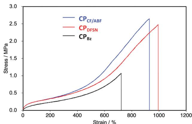
Fig. 5 Stress–strain curves of  $\text{CP}_{\text{CF/ABF}}$  (blue),  $\text{CP}_{\text{DFSN}}$  (red) and  $\text{CP}_{\text{Bz}}$  (black) films ( $100 \text{ mm min}^{-1}$ ,  $30 \text{ }^\circ\text{C}$ ).
