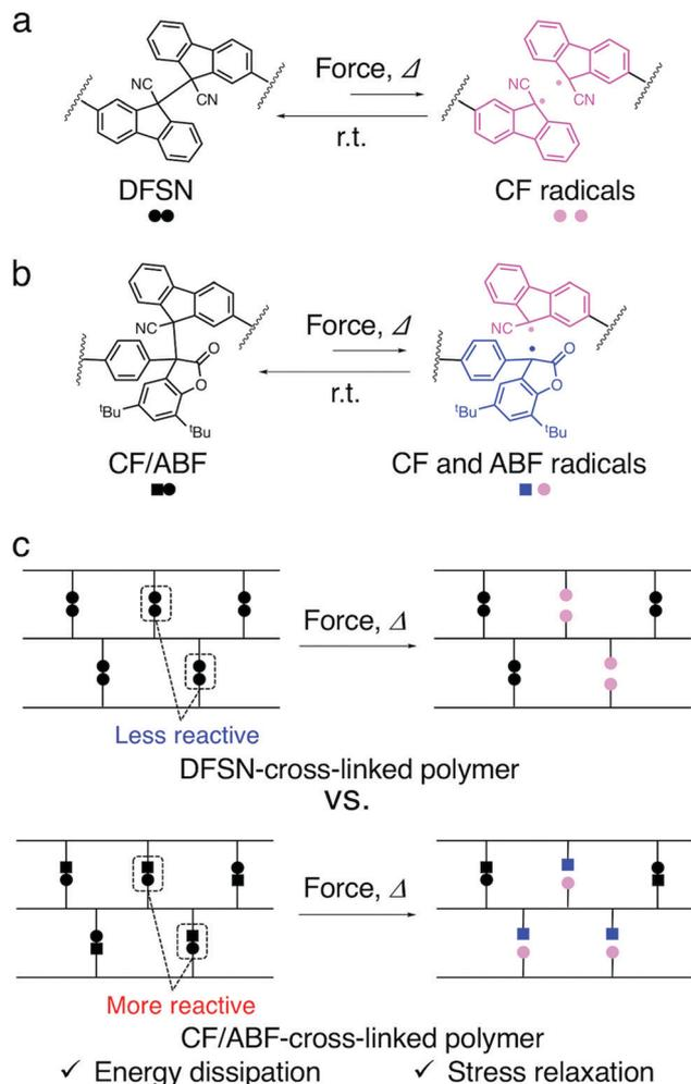
**Fig. 1** (a) Equilibrium between DFSN and its radical species. (b) Equilibrium between CF/ABF and its radical species. Illustration of (c) a DFSN-cross-linked polymer and a CF/ABF-cross-linked polymer, as well as the mechanism of energy dissipation and stress relaxation.
