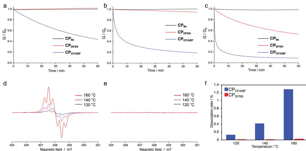
Fig. 3 Stress-relaxation behavior of **CP<sub>x</sub>** at (a) 120, (b) 140 and (c) 160 °C. EPR spectra of (d) **CP<sub>CF/ABF</sub>** and (e) **CP<sub>DFSN</sub>** at 120, 140 and 160 °C. (f) Dissociation ratio of CF/ABF and DFSN in **CP<sub>CF/ABF</sub>** and **CP<sub>DFSN</sub>** at 120, 140 and 160 °C.
