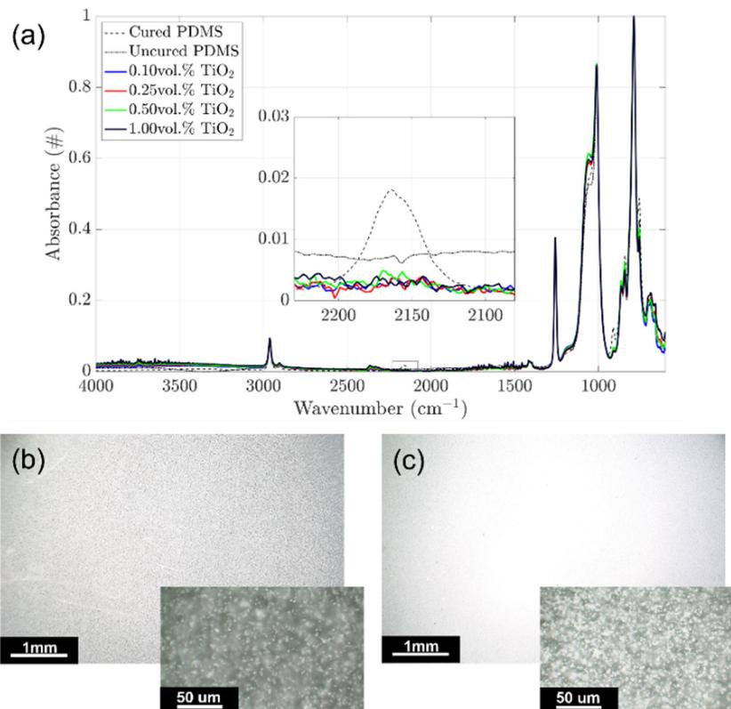
Fig. 1 (a) FT-IR ATR spectra focused on the Si-H reacting groups ( $2160 \text{ cm}^{-1}$ ) at increasing  $\text{TiO}_2$  particle concentrations (0, 0.1, 0.25, 0.5, and 1 vol%). Optical microscopy images taken at increasing magnifications of PDMS with 0.25 (b) and 1 (c) vol%  $\text{TiO}_2$ .
