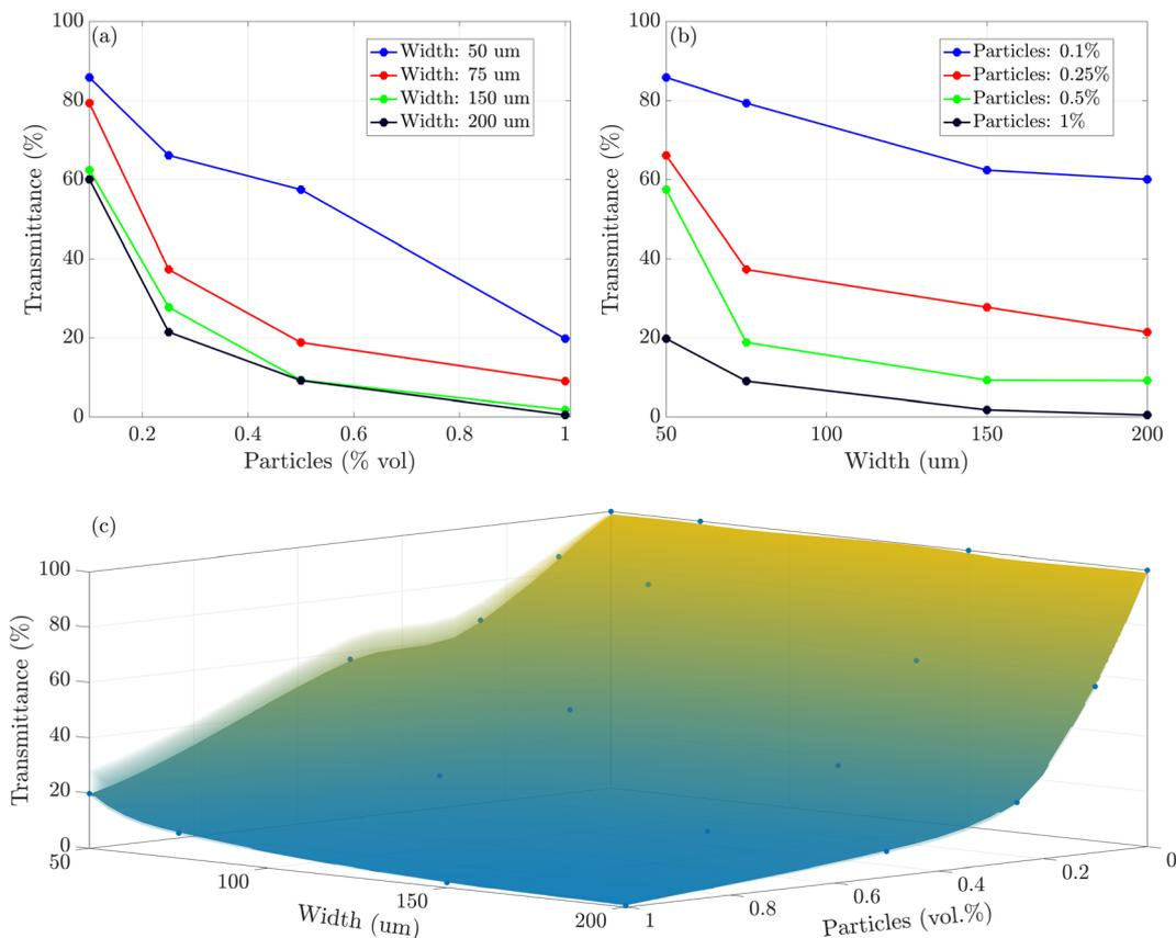
Fig. 3 (a) Effect of the  $\text{TiO}_2$  concentration in the NIR transmittance for constant film thickness. (b) Effect of the film thickness on the NIR transmission for constant  $\text{TiO}_2$  concentrations. (c) Combination of the  $\text{TiO}_2$  concentration and the film thickness on the light transmission. All the graphs refer to 850 nm wavelength.
