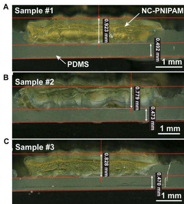
Fig. 3 Optical microscope photographs of the cross-sectional view of the hinge-based bilayer structure of NC-PNIPAM/PDMS printed with the target thickness ( $h_1 = 0.6$  mm,  $h_2 = 0.4$  mm). (A) Sample #1 with  $h_1 = 0.923$  mm,  $h_2 = 0.492$  mm; (B) sample #2 with  $h_1 = 0.779$  mm,  $h_2 = 0.473$  mm; (C) sample #3 with  $h_1 = 0.828$  mm,  $h_2 = 0.470$  mm.
