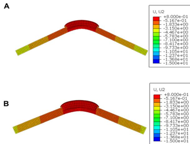
Fig. 4 The simulated folding structure using the (A) target thickness = 0.6 mm,  $h_2 = 0.2$  mm and (B) actual thickness ( $h_1 = 0.779$  mm,  $h_2 = 0.473$  mm). Color bars shown on the right indicate the simulated displacement in the vertical direction.
