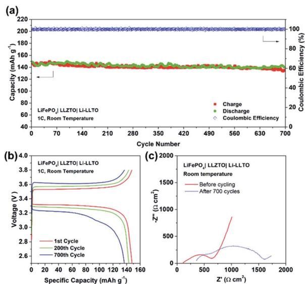
Fig. 8 The overall SSB cycling performance. (a) Cycling performance of  $\text{LiFePO}_4$ |LLZTO|Li-LLTO at a rate of 1C at room temperature. (b) Charge and discharge curves for the 1<sup>st</sup>, 200<sup>th</sup>, and 700<sup>th</sup> cycles at 1C. (c) EIS curves of the fresh cell and cycled cell for the  $\text{LiFePO}_4$ |LLZTO|Li-LLTO SSB.
