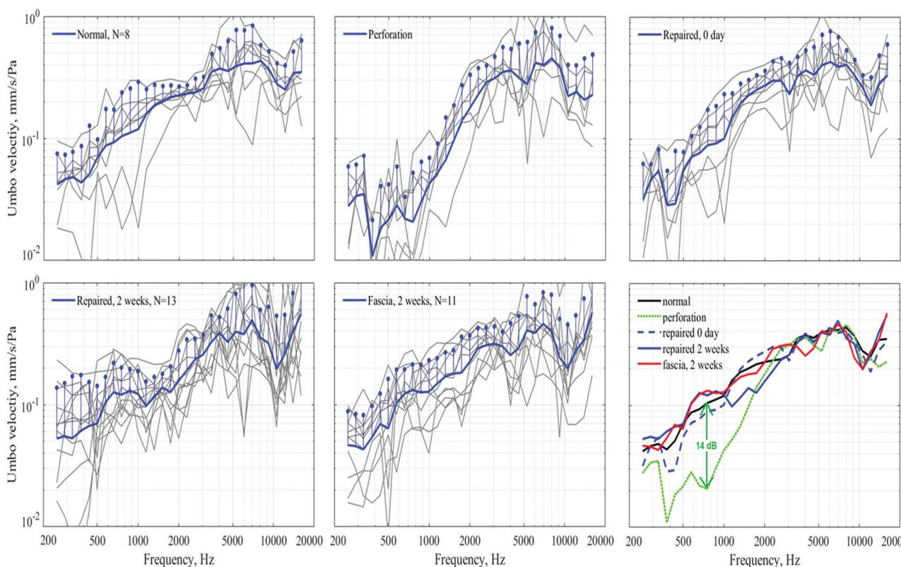
Fig. 5 Umbo velocities of TM of different states.
