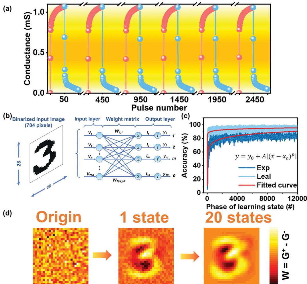
Fig. 4 (a) Use 25-cycle pulses (50 positives (4 V) and 50 negatives (−2 V) pulses with a pulse duration of 50 ms and an interval of 50 ms) to simulate the synaptic TFT channel conductance. (b) ANN structure used in the simulation. (c) Simulation of MNIST digit recognition accuracy based on synaptic TFT perceptron neural network. (d) Mapping images of test data sets for three different learning epochs.
