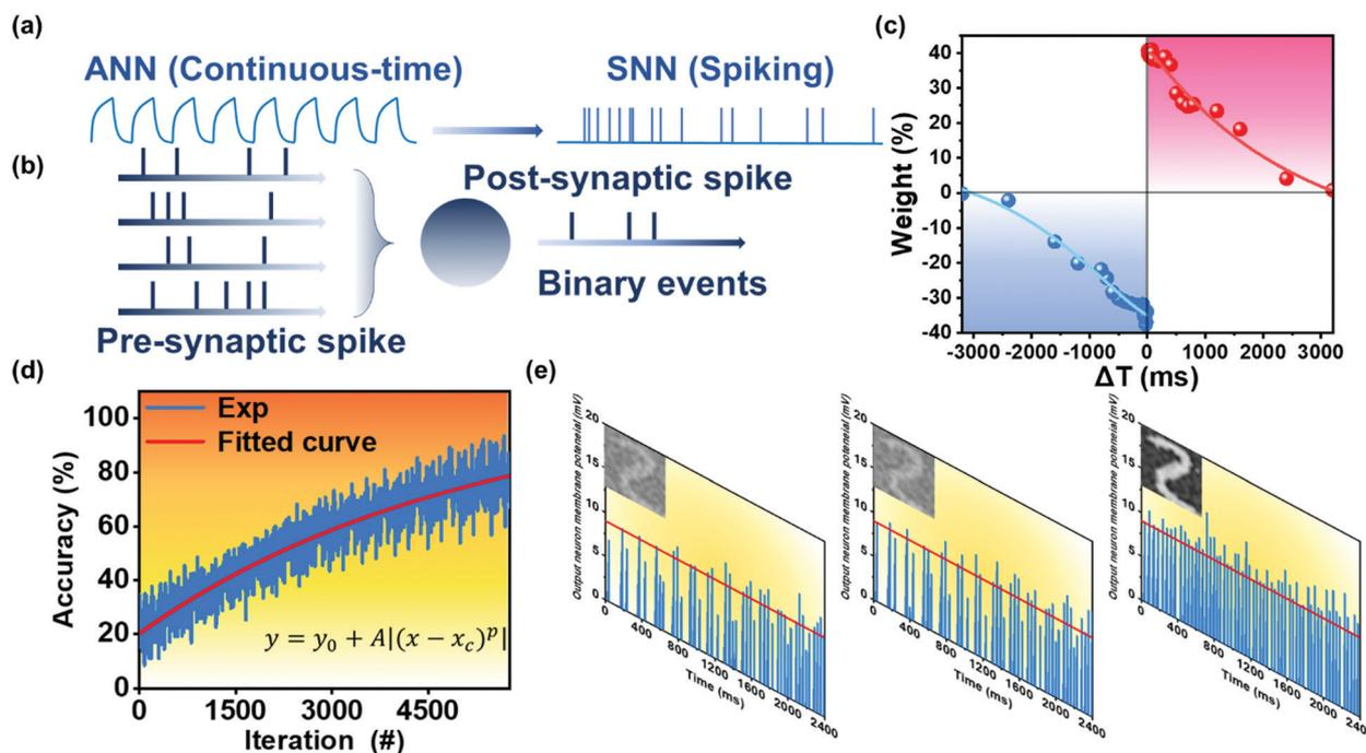
Fig. 5 (a) ANN algorithm and SNN algorithm function diagram. (b) SNN algorithm weight update diagram. (c) STDP response based on  $K^+$  doped  $AlO_x$  synaptic devices. (d) Image recognition rate of SNN algorithm. (e) Different stage results of training the SNN using the MNIST data set. Via the generation characteristics of the SNN, the image is reconstructed using the training weights connected to each output neuron to view the learning situation of the network.
