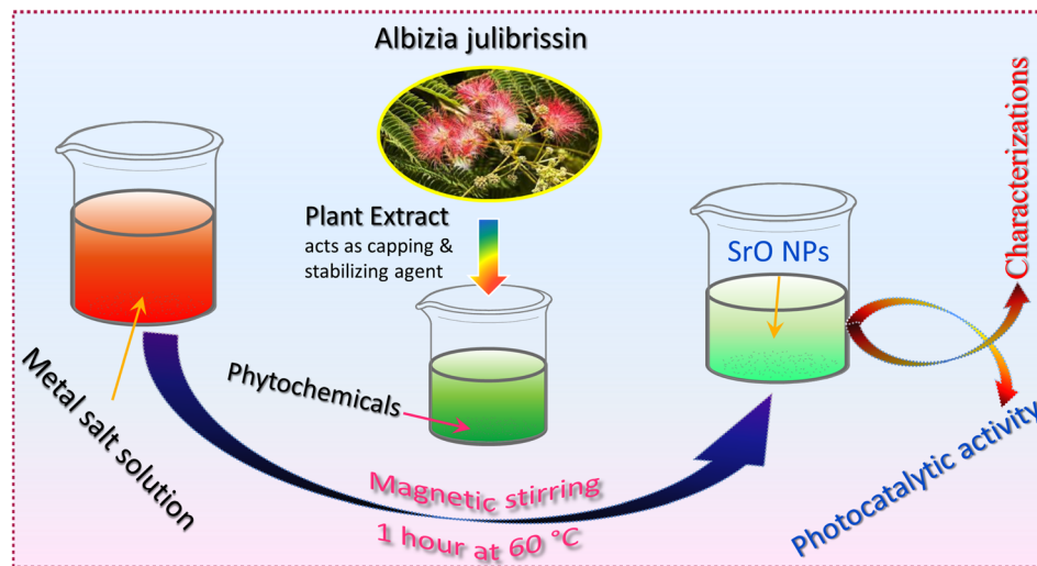
Scheme 1 Schematic illustration of the green synthesis procedure for SrO nanoparticles.
