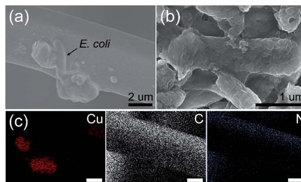
Fig. 5 (a) Scanning electron microscopy (SEM) image showing the surface interaction between *E. coli* and Cu NPs in Cu/MS, (b) SEM image showing a ruptured *E. coli* cell and (c) SEM and the corresponding elemental mapping showing the surface interaction between *E. coli* and Cu NPs in Cu/MS by EDS analysis: Cu (red), N (blue), O (yellow), and C (gray).
