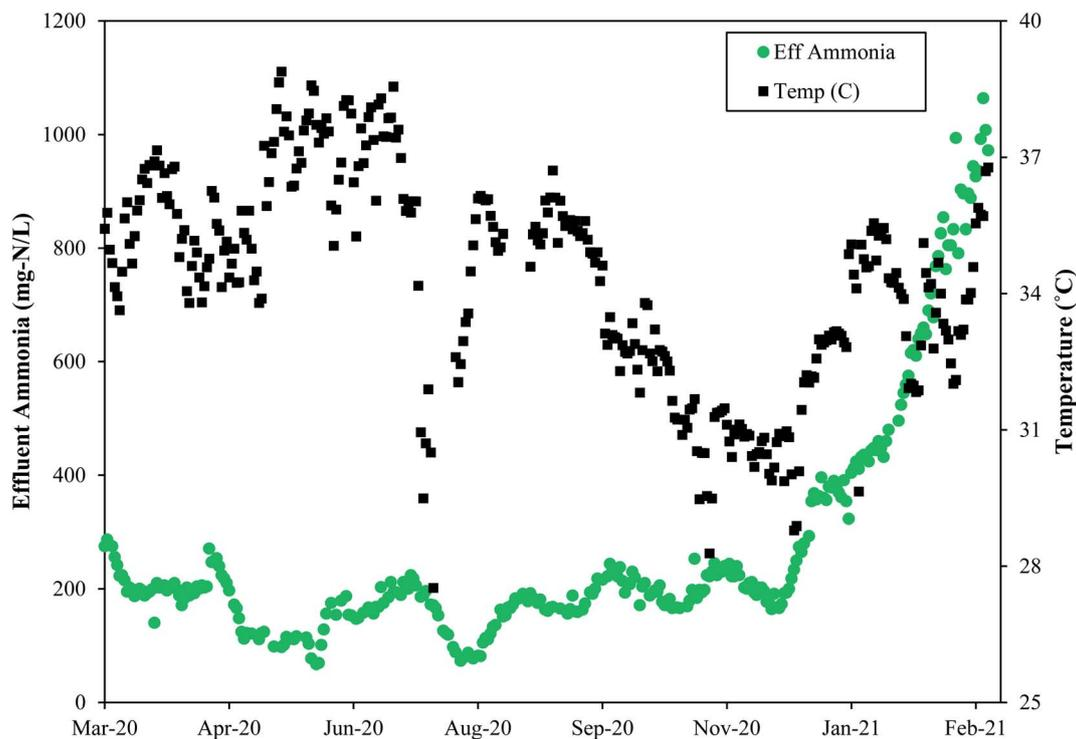
Fig. 5 The temperature drops near the end of 2020 preceded the major process upset as evidenced by the rise in effluent ammonia concentrations at the Denver NTP.
