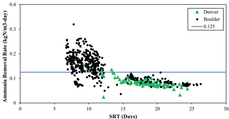
Fig. 1 The impact of SRT on ammonia removal rates. The blue line is 0.125 kgN m<sup>-3</sup>-day and is used to distinguish between “low” and “high” ammonia removal rates.
