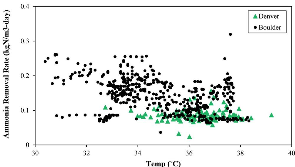
Fig. 4 Impact of temperature on ammonia removal rate.
