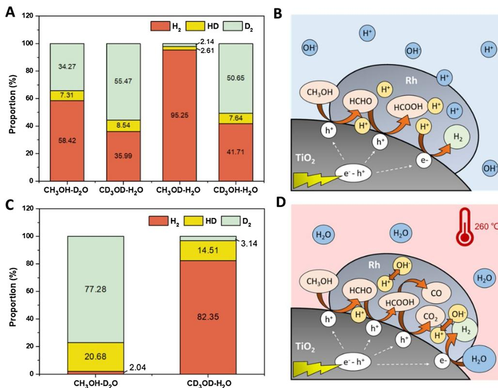
Fig. 7 Results from isotopic labelling experiments (A and C) and schematic process representation of the reaction mechanism (B and D) of a Ru/TiO<sub>2</sub> catalyst using a methanol:water mixture. Thermo (A and B) and thermo-photo (C and D) conditions are tested. Reproduced with permission from ref. 67. Copyright Elsevier.
