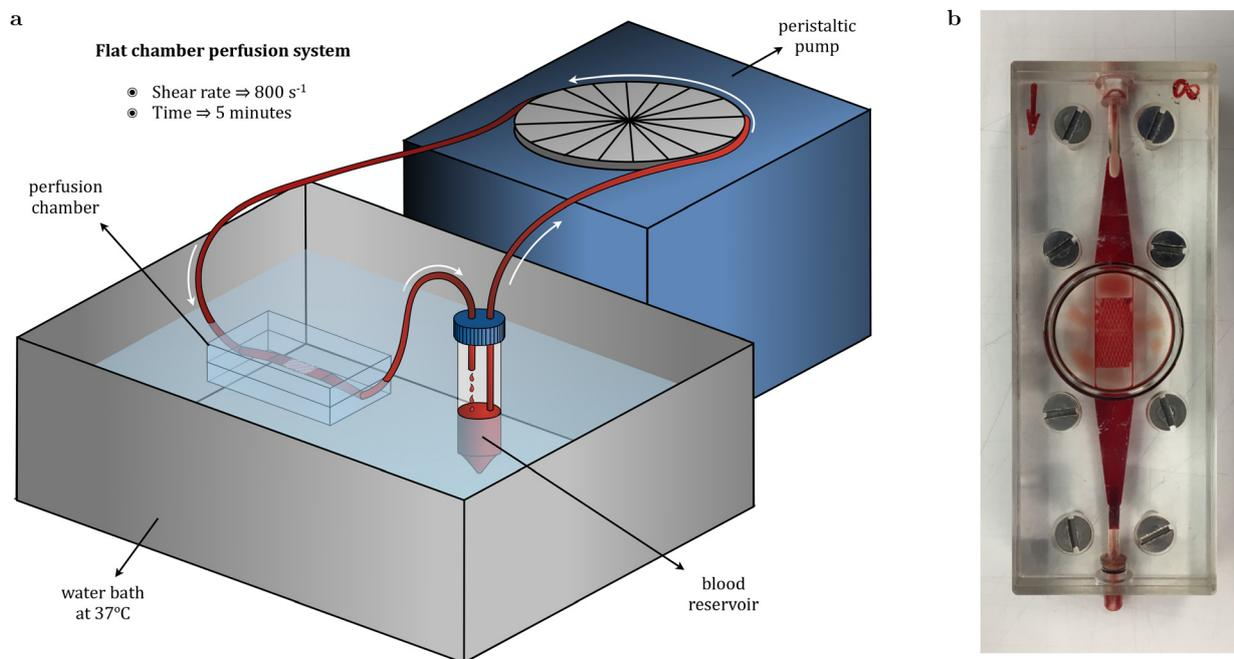
**Fig. 2** (a) Scheme showing the experimental setup used for the thrombogenicity assay. Blood from a healthy donor was circulated through the stent in the perfusion chamber at a shear rate of  $800 \text{ s}^{-1}$  for 5 minutes using a peristaltic pump. Both the blood reservoir and the perfusion chamber were maintained in a water bath at  $37^\circ\text{C}$ . (b) Detail of the perfusion chamber after the assay, with the stent aligned with the blood flow.
