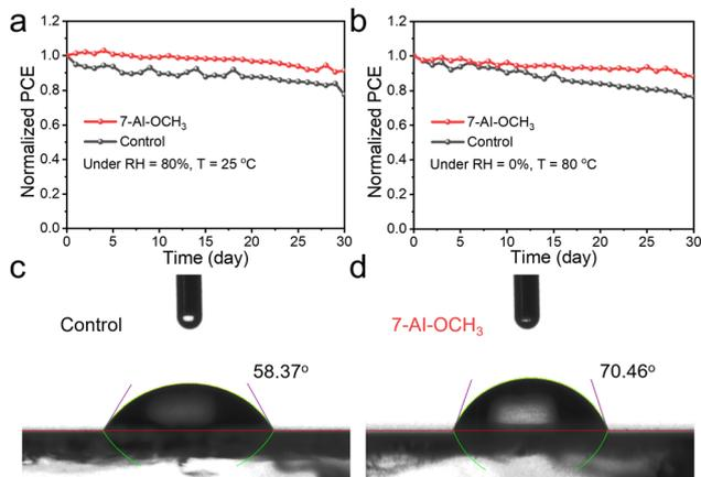
Fig. 4 Long-term stability of the inorganic CsPbBr<sub>3</sub> PSCs at (a) RH = 80%, T = 25 °C and (b) RH = 0%, T = 80 °C. The water contact angle of (c) control and (d) 7-Al-OCH<sub>3</sub>-based perovskite films.
