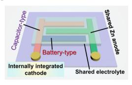
Design of internally integrated in-plane electrodes for superior flexible hybrid zinc-ion capacitor devices
