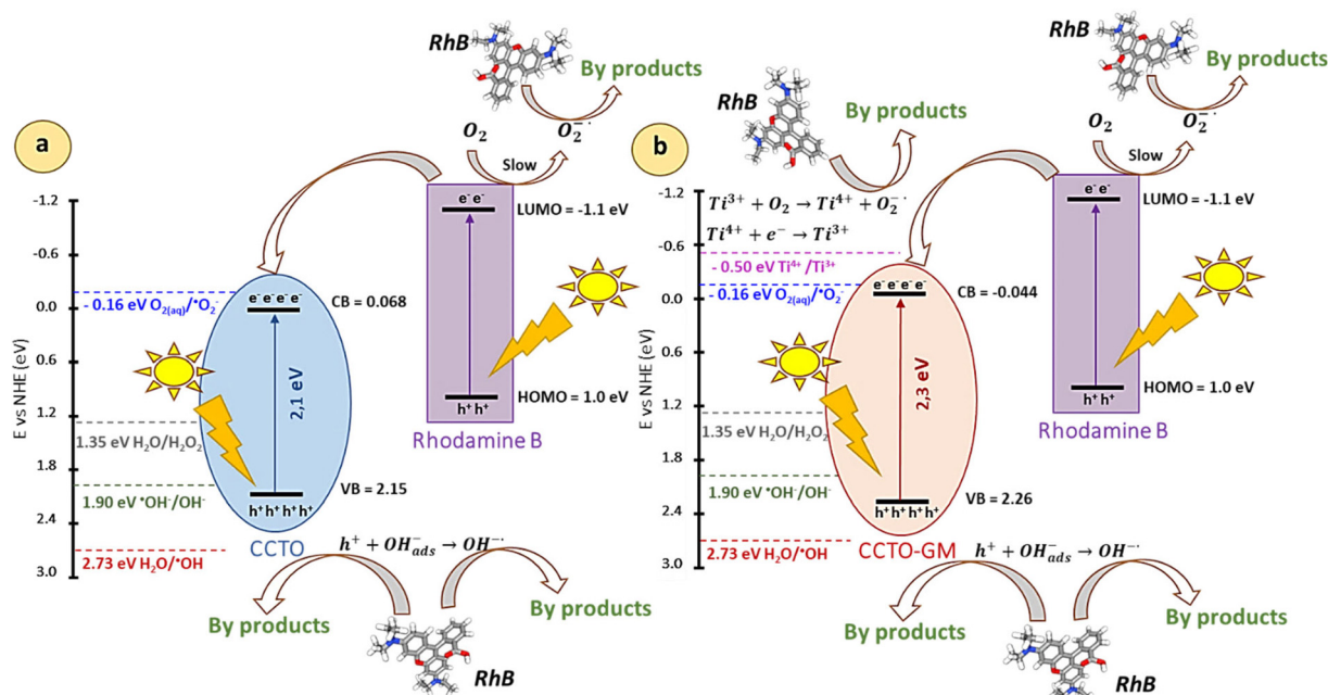
Fig. 13 Schematic representation of solar light driven degradation mechanisms of rhodamine B by a) CCTO, b) CCTO-GM.
