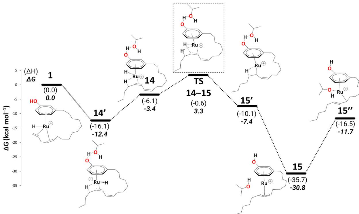
**Scheme 8** Reduction to the monoene: from intermediate **14'** to **15'** (B3PW91-D3BJ/ECP2/PCM level, iPrOH as the model solvent with enthalpic and entropic corrections at 355.65 K). Energies ( $\Delta H$  and  $\Delta G$ ) are in kcal mol<sup>-1</sup> relative to **1**. The wavy line represents multiple steps. Table S3† shows the reaction energies of individual steps.
