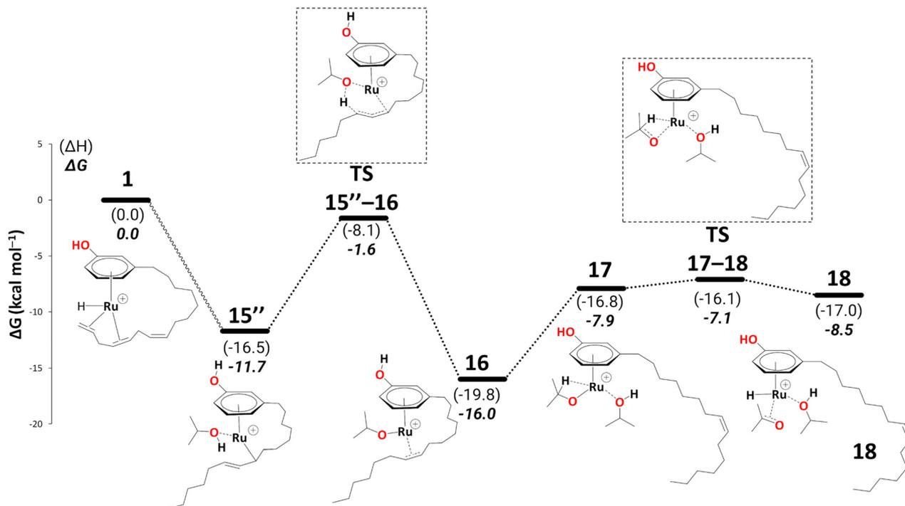
**Scheme 9** Reduction to the monoene: from intermediate 15'' to 18 (B3PW91-D3BJ/ECP2/PCM level, iPrOH as the model solvent with enthalpic and entropic corrections at 355.65 K). Energies ( $\Delta H$  and  $\Delta G$ ) are in kcal mol<sup>-1</sup> relative to 1. The wavy line represents multiple steps. Table S3 shows the reaction energies of individual steps.
