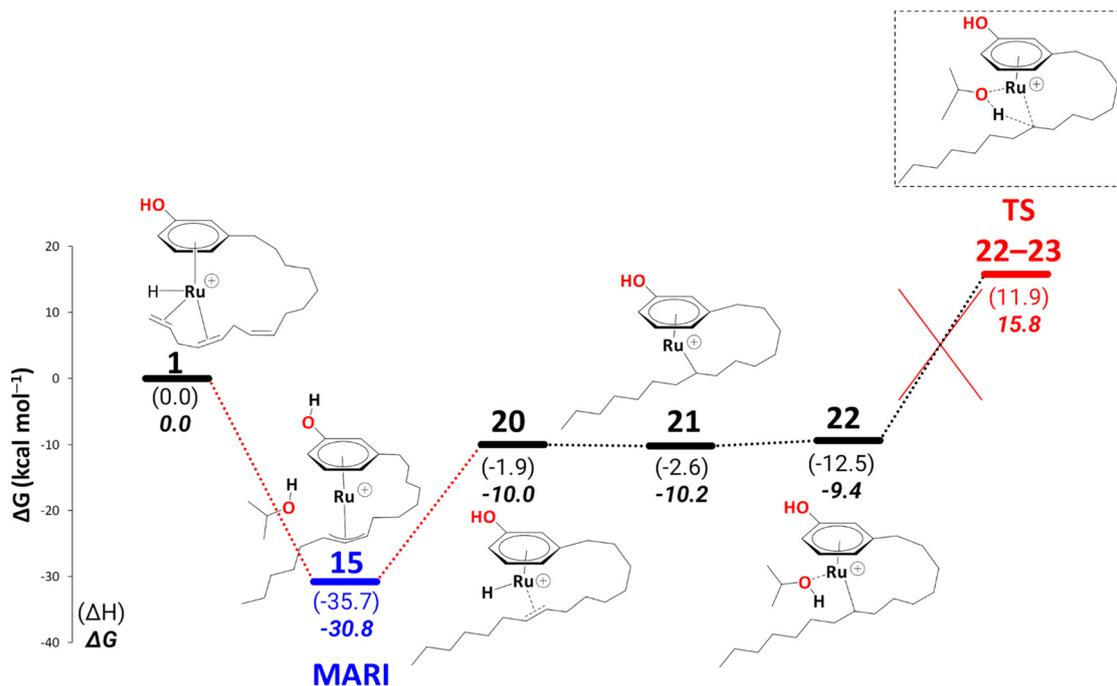
**Scheme 13** Reduction to the fully saturated cardanol derivative at the B3PW91-D3BJ/ECP2/PCM level with *i*PrOH as the model solvent with enthalpic and entropic corrections at 355.65 K. Energies ( $\Delta H$  and  $\Delta G$ ) are in  $\text{kcal mol}^{-1}$  relative to **1**. The red dotted lines represent multiple steps. Table S4<sup>†</sup> shows the reaction energies of individual steps.
