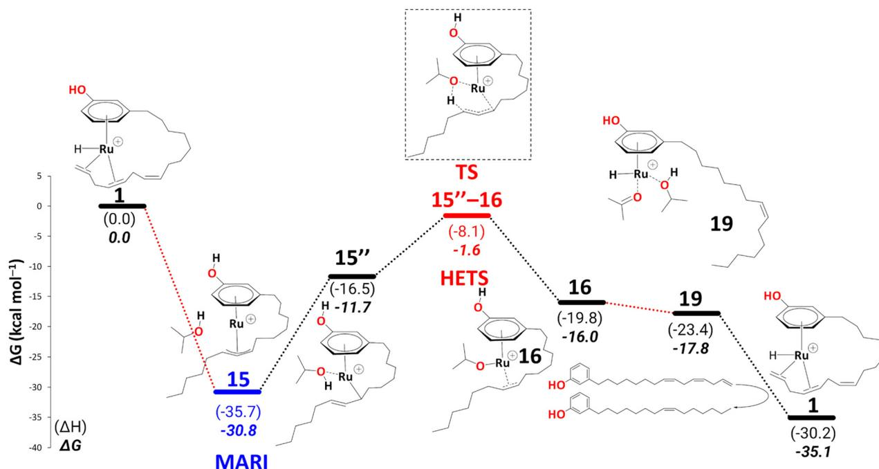
**Scheme 12** Reduction to the cardanol monoene: key intermediates and transition state are shown, with **15** as MARI and **TS15–16** as HETS. Energies ( $\Delta H$  and  $\Delta G$ ) are calculated at B3PW91-D3BJ/ECP2/PCM level with iPrOH as the model solvent with enthalpic and entropic corrections at 355.65 K relative to **1**. The red dotted lines represent multiple steps.
