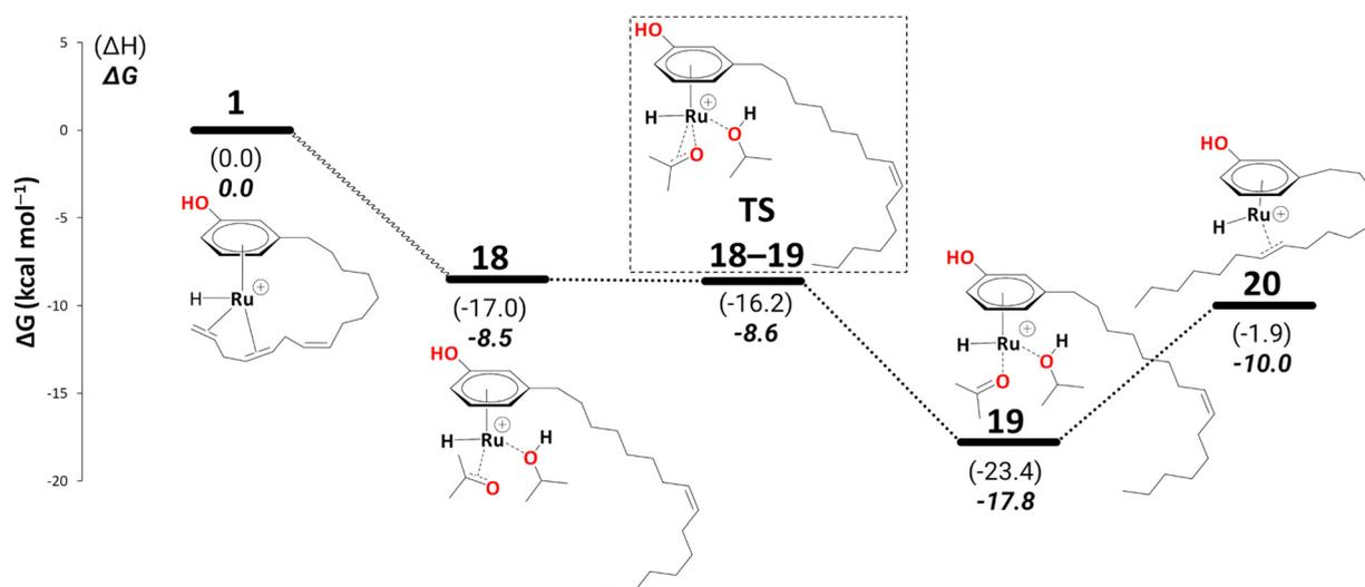
**Scheme 10** Reduction to the monoene: from intermediate 18 to 20 (B3PW91-D3BJ/ECP2/PCM level, iPrOH as the model solvent with enthalpic and entropic corrections at 355.65 K). Energies ( $\Delta H$  and  $\Delta G$ ) are in kcal mol<sup>-1</sup> relative to 1. The wavy line represents multiple steps. Table S3† shows the reaction energies of individual step.
