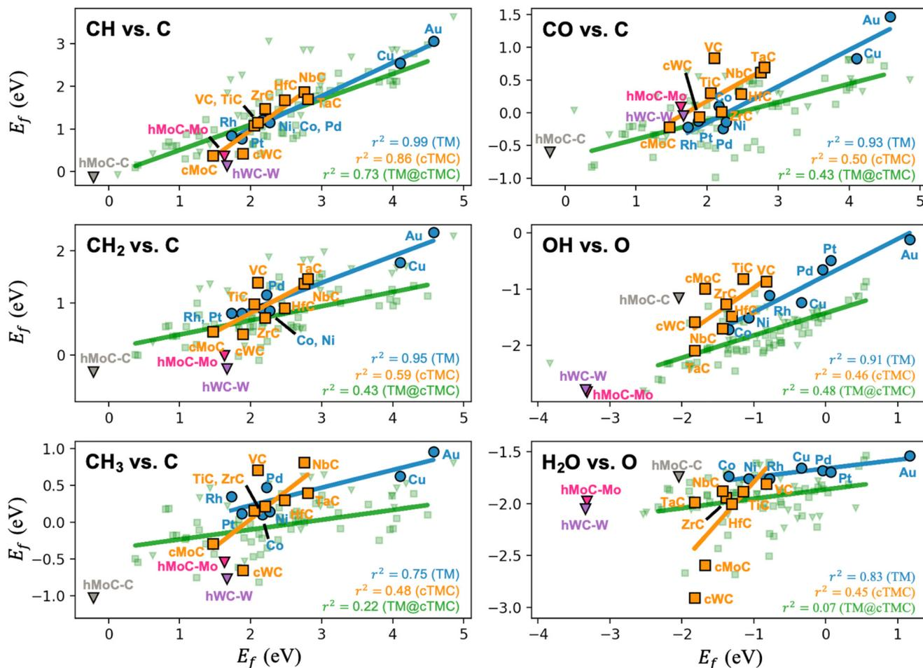
Fig. 3 Linear scaling plots between the formation energies of different adsorbates on TMs, TMCs and  $TM_n@TMCs$ . Trend lines and  $R$ -squared coefficients are included. Note that hexagonal TMCs (shown as triangles) have been excluded from the TMC trend lines, as they exhibit different adsorption sites compared to cubic TMCs. All other linear scaling plots for TM and TMC are shown in Fig. S7 and S8<sup>†</sup> respectively.
