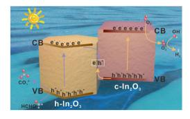
Enhanced adsorption of oxygen species on c/h-In<sub>2</sub>O<sub>3</sub> Z-scheme heterophase junctions for oxygenmediated photocatalytic hydrogen production
