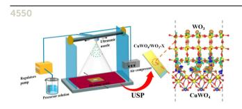
Interfacial engineering of CuWO<sub>4</sub>/WO<sub>3</sub> thin films precisely fabricated by ultrasonic spray pyrolysis for improved solar water splitting
