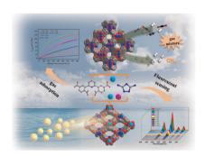
A gas-selective Zn-MOF exhibits selective sensing of Fe<sup>3+</sup> ions by doping with Tb<sup>3+</sup>
