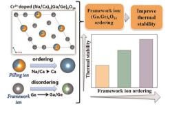
Influence of framework disordering on the luminescence performance of  ${\rm Cr}^{3+}$ -doped near-infrared phosphors: a case study of  ${\rm A_3B_6O_{14}}$ -type hosts
