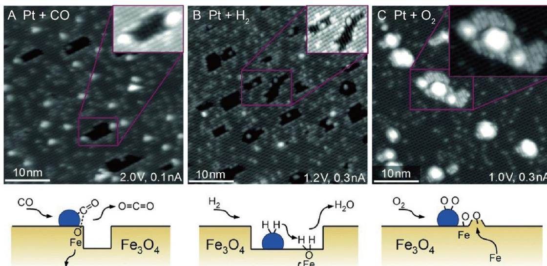
**Fig. 10** STM images acquired following exposure of the Pt/Fe<sub>3</sub>O<sub>4</sub>(001) model catalyst to  $1 \times 10^{-7}$  mbar (A) CO, (B) H<sub>2</sub>, and (C) O<sub>2</sub> at 550 K. Reproduced with permission.<sup>69</sup> Copyright © 2015 WILEY-VCH Verlag GmbH & Co. KGaA, Weinheim.
