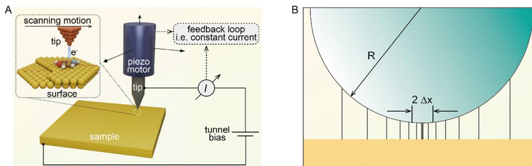
Fig. 1 (A) Simplified basic set-up for STM. Reproduced with permission.<sup>3</sup> Copyright © 2021, Springer Nature Limited. (B) Estimation of the lateral resolution in STM. Reproduced with permission.<sup>4</sup> Copyright © 1993, Oxford University Press.
