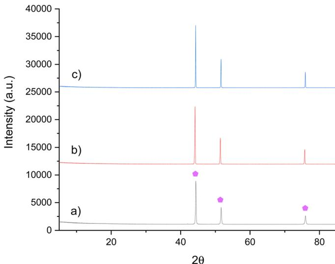
Fig. 11 XRD patterns of Ni<sub>3</sub>Cu: (a) pre N<sub>2</sub> treatment, (b) post N<sub>2</sub> treatment at 700 °C and (c) post N<sub>2</sub> treatment at 800 °C. (⬠) Ni<sub>3</sub>Cu.
