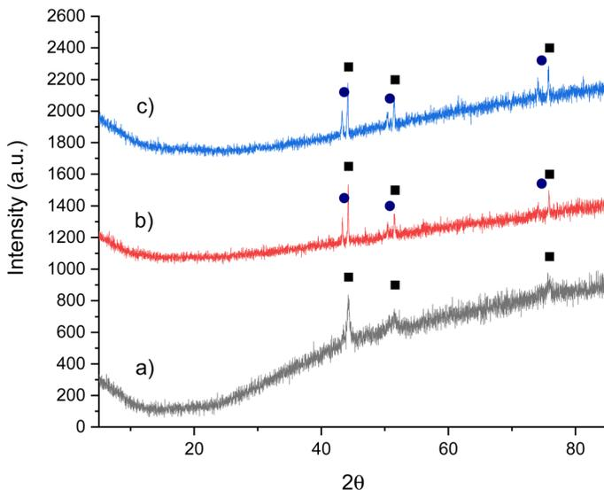
Fig. 6 XRD patterns of  $\text{Co}_3\text{Cu}$ : (a) pre  $\text{N}_2$  treatment, (b) post  $\text{N}_2$  treatment at  $700\text{ }^\circ\text{C}$  and (c) post  $\text{N}_2$  treatment at  $800\text{ }^\circ\text{C}$ . (■)  $\text{Co}_3\text{Cu}$  and (●) Cu.
