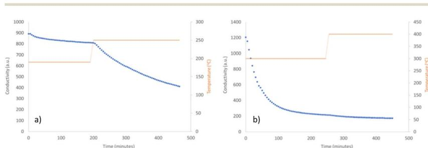
Fig. 3 Ammonia production reaction profiles of  $\text{Co}_3\text{CuN}$  reacted with  $60 \text{ mL min}^{-1}$  of 3 : 1  $\text{H}_2/\text{N}_2$  (a) for 3 hours at 200 °C and 4 hours 25 minutes at 250 °C and (b) for 4 hours at 300 °C and 3 hours 15 minutes at 400 °C.
