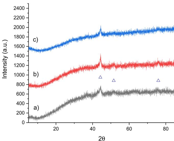
Fig. 16 XRD patterns of  $\text{Co}_3\text{MoN}$ : (a) pre-reaction, (b) post-reaction with 3 : 1  $\text{H}_2/\text{N}_2$  at 200 °C and 250 °C and (c) post-reaction with 3 : 1  $\text{H}_2/\text{N}_2$  at 300 °C and 400 °C. (Δ) Co.
