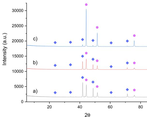
Fig. 7 XRD patterns of Ni<sub>3</sub>CuN: (a) pre-reaction, (b) post-reaction with 3 : 1 H<sub>2</sub>/N<sub>2</sub> at 250 °C and (c) post-reaction with 3 : 1 H<sub>2</sub>/N<sub>2</sub> at 300 °C and 400 °C. (◆) Ni<sub>3</sub>CuN and (◻) Ni<sub>3</sub>Cu.
