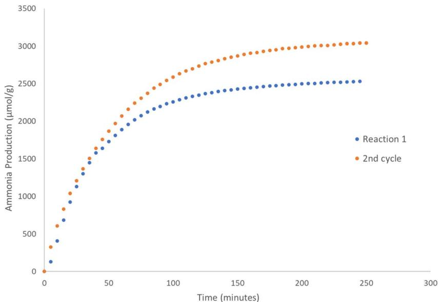
Fig. 5 Ammonia production reaction profiles of the 1st and 2nd cycles for  $\text{Co}_3\text{CuN}$  reacted with  $60 \text{ mL min}^{-1}$  of 3:1  $\text{H}_2/\text{N}_2$  at  $300^\circ\text{C}$  for 4 hours.
