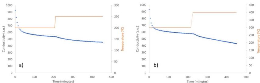
Fig. 18 Ammonia production reaction profiles of 'Co<sub>3</sub>MoN' reacted with 60 mL min<sup>-1</sup> of 3 : 1 H<sub>2</sub>/N<sub>2</sub> (a) for 3 hours 25 minutes at 200 °C and 4 hours 5 minutes at 250 °C and (b) for 3 hours 35 minutes at 300 °C and 3 hours 45 minutes at 400 °C.
