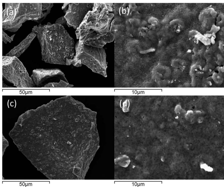
Fig. 8 Representative SEM images of Ni<sub>3</sub>CuN: (a and b) pre-reaction and (c and d) post N<sub>2</sub>/H<sub>2</sub> reaction at 300 °C and 400 °C.
