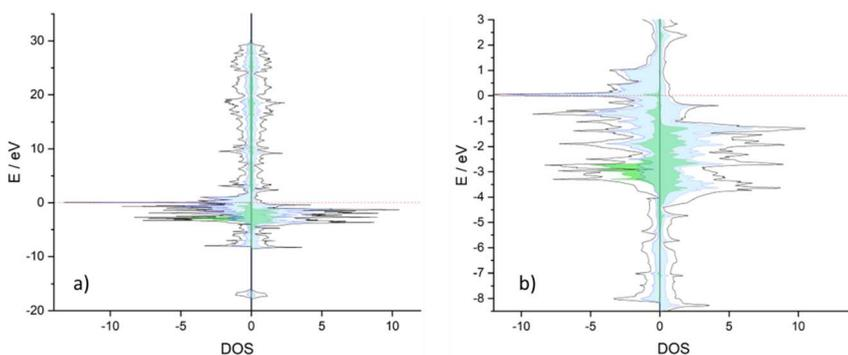
Fig. 15 Plots for the projected density of states (DOS) for  $\text{Co}_3\text{CuN}$ : (a) full DOS and (b) highlighted area for metal d states at the Fermi level. Black lines: total DOS, shaded blue: Co and shaded green: Cu.
