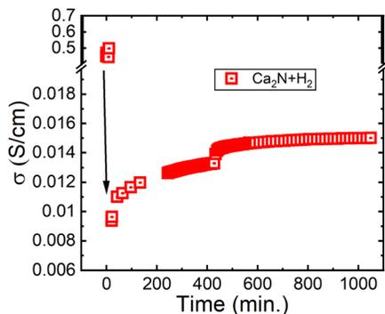
Fig. 4 EIS calculated conductivity from  $\text{Ca}_2\text{N}$  exposed to 5%  $\text{H}_2$  in Ar at 600 °C. The initial conductivity is for the  $\text{Ca}_2\text{N}$  phase, while the resulting conductivity is from  $\text{Ca}_2\text{NH}$  as shown by the post experiment XRD pattern 1 (see Fig. 1b).
