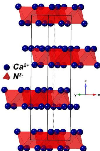
Fig. 2 Crystal model of  $\text{Ca}_2\text{N}$  showing Ca–N octahedra. Electrons are thought to exist between the layers.<sup>17</sup>
