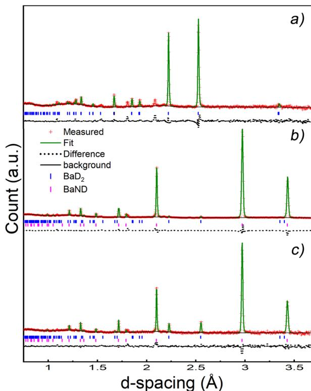
Fig. 9 NPD patterns: (a) starting pattern refined with the HT BaD<sub>2</sub> phase. (b) Pattern 120 (*i.e.* the middle of the experiment) refined with a HT BaD<sub>2</sub> phase and a BaND phase. The refinement gave an 80% concentration of BaND by weight. (c) Last 73 patterns summed and refined with a BaD<sub>2</sub> and BaND phase. The refinement gave a 96% concentration of BaND by weight.
