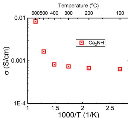
Fig. 6 Log of conductivity plot for the Ca<sub>2</sub>NH system. A large jump in conductivity is observed between 400 and 500 °C. A similar jump was observed in the H<sup>-</sup> conductor Ba<sub>2</sub>NH by Altorfer *et al.*<sup>26</sup>
