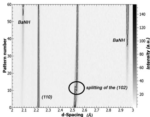
Fig. 8 Contour plot showing the evolution of NPD patterns versus pattern number (each pattern is  $\sim 2$  min). After 20 min of exposure to  $N_2$ , the (102) reflection of  $BaD_2$  splits, while the (110) peak remains unchanged. The emergence of a second phase is clear at pattern number 40 (80 min).
