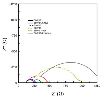
Fig. 5 EIS data collected on a  $\text{Ca}_2\text{N}$  pellet exposed to  $\text{H}_2$  gas at varying temperatures. Data is in chronological order. The data shows that the arc associated with a surface layer ( $10^{-9}$  to  $10^{-7} \text{ F}^{21}$ ) doubles after two days at 600 °C. The grey spectrum shows the data collected at 600 °C used for the conductivity log plot (see Fig. 6).
