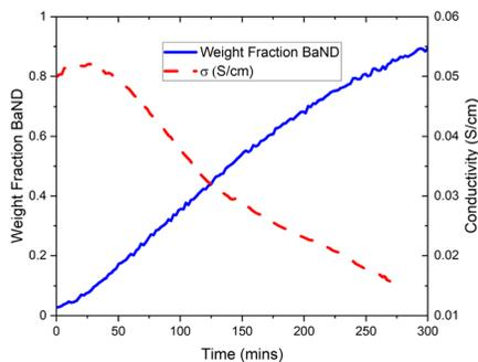
Fig. 10 Trend in calculated conductivity and phase fraction of BaND for doping of BaD<sub>2</sub> with N<sub>2</sub> experimentally. The emergence of BaND is associated with a decrease in conductivity. Beyond 280 min, the resistance associated with the high frequency response increases dramatically making the accurate modelling of the  $R_s$  difficult.
