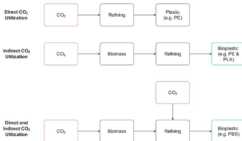
Fig. 4 Indirect and direct utilization of CO<sub>2</sub> for polymer production. PE = polyethylene, PLA = polylactic acid, PBS = polybutylene succinate.
