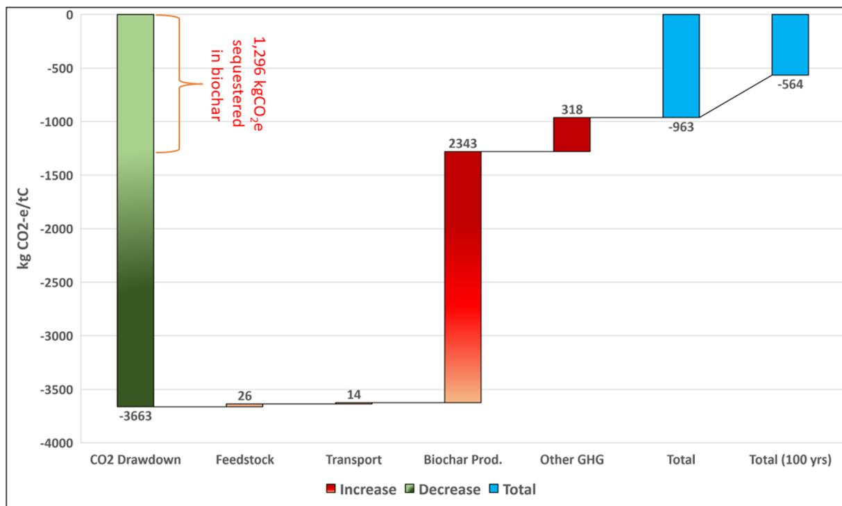
**Fig. 10** Biochar soil amendment drawdown over 100 years (moderate case). Note that in the waterfall diagrams, green and red bars represent magnitudes of drawdown and emissions subsequent to the initial drawdown in biomass. The blue bars represent totals. The sum of all red and green bars is equal to the first blue bar.
