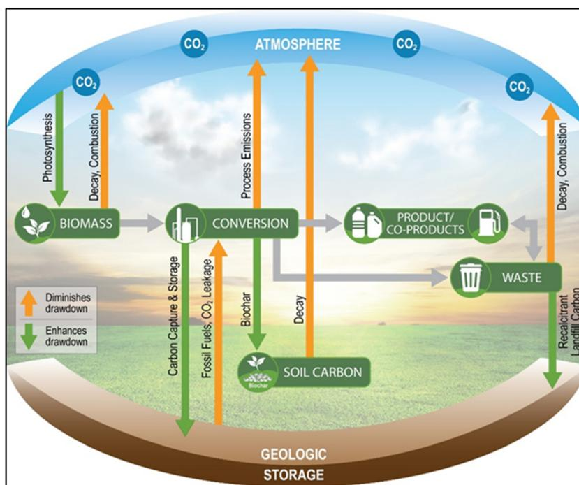
**Fig. 1** Carbon flows associated with carbon drawdown from bioproducts. To enhance carbon drawdown, the flows represented by the green arrows need to increase in magnitude while minimizing the flows represented by the orange arrows. The grey arrows represent biogenic carbon moving through the bioeconomy life cycle while the orange and green arrows indicate carbon losses and storage, respectively.
