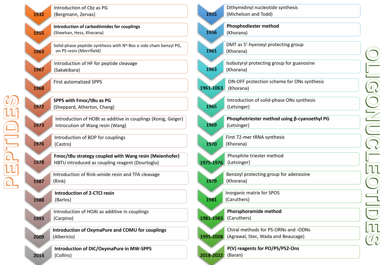
Fig. 2 The 14 most relevant updates on the solid-phase synthesis of TIDES.
