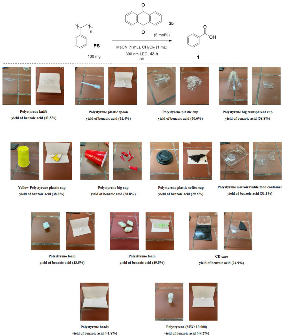
Scheme 4 Photochemical aerobic upcycling of commercially available PS products and daily life PS wastes (left: PS-derived plastic object, right: cut Ps-based plastic pieces, in order to be employed as the reaction substrate).
