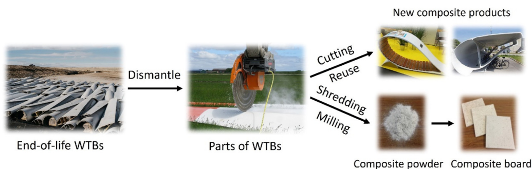
Fig. 4 Mechanical recycling processes of end-of-life WTBs.
