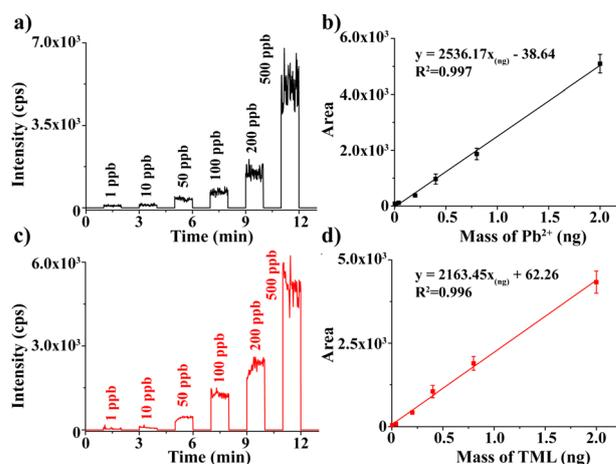
Fig. 3 Quantitative analysis of  $\text{Pb}^{2+}$  and TML by EC-MS. EIC of (a)  $\text{Pb}^{2+}$  and (c) TML calibration solution with different concentrations. The EIC area of (b)  $\text{Pb}^{2+}$  and (d) TML against the corresponding mass ( $n = 3$ ).
