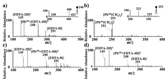
Fig. 2 Mass spectra of Pb components in different speciations analyzed by EC-MS. (a)  $\text{Pb}(\text{NO}_3)_2$ , (b) TML, (c)  $\text{PbCO}_3$  and (d) Pb. The insets were the MS/MS spectrum of the isolated ions.
