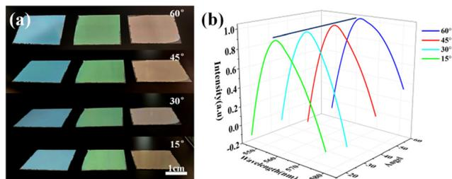
**Fig. 2** Angle-independent structural color of the APS/Ag film. (a) Photos of three structural colored films produced by the hand-writing method at viewing angles of 60°, 45°, 30° and 15°. (b) Reflection spectra of the green film at viewing angles of 60°, 45°, 30° and 15°. The viewing angles refer to the angles between the reflected light and the horizontal plane.
