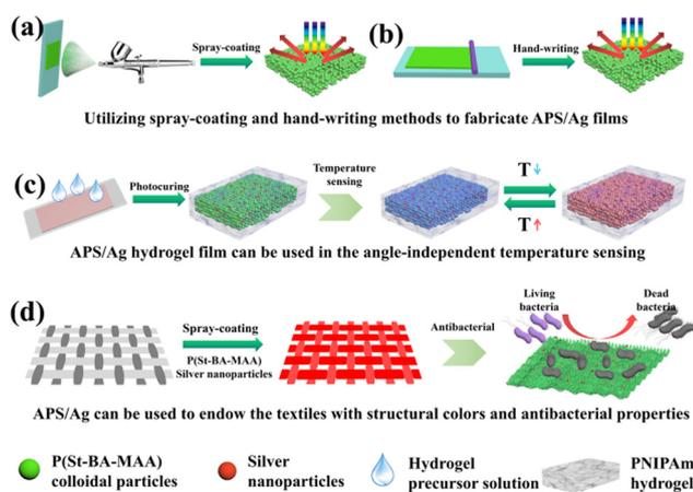
**Scheme 1** Facile fabrication of APS films with noniridescent structural colors by doping Ag NPs utilizing the methods of (a) spray-coating and (b) hand-writing. (c) Schematic illustration of the preparation of the Ag NP-doped temperature sensor produced by embedding the colloidal particles in the NIPAm hydrogel. (d) Antibacterial textiles constructed by the spray-coating method.
