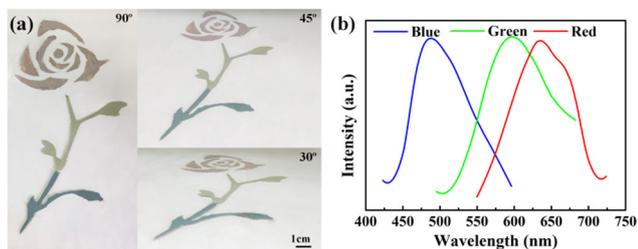
**Fig. 3** A colorful structural color pattern constructed on PET film by the hand-writing method. (a) The pattern of a 'rose' at viewing angles of 60°, 45° and 30°. (b) Reflection spectra of three colors. The viewing angles refer to the angles between the reflected light and the horizontal plane.
