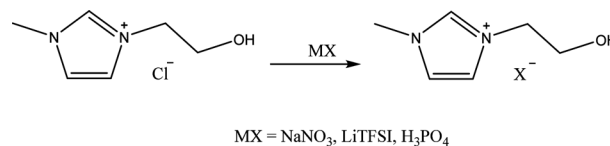
Scheme 1 Synthesis of hydroxyl [ILs-OH] + [X] - with different anions.
