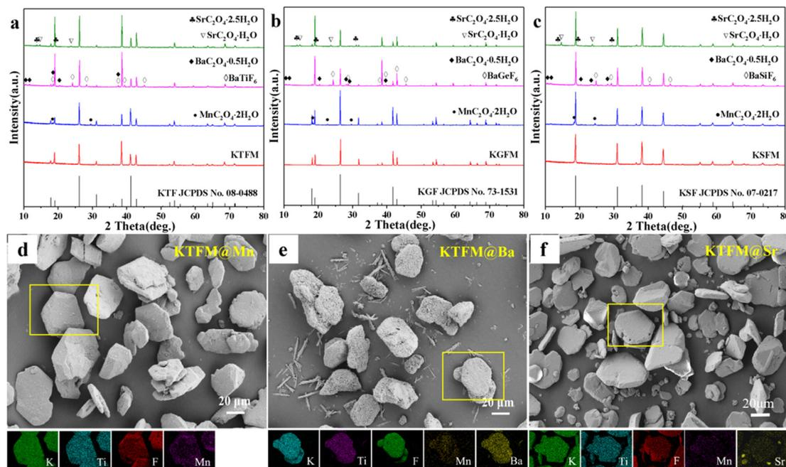
Fig. 2 (a)–(c) XRD patterns of  $\text{MC}_2\text{O}_4$  ( $M = \text{Sr}, \text{Ba}, \text{Mn}$ ) modified  $\text{K}_2\text{XF}_6:\text{Mn}^{4+}$  ( $X = \text{Ti}, \text{Ge}, \text{Si}$ ). (d)–(f) SEM and EDS mapping images of  $\text{MC}_2\text{O}_4$  ( $M = \text{Sr}, \text{Ba}, \text{Mn}$ ) modified  $\text{K}_2\text{TiF}_6:\text{Mn}^{4+}$ .
