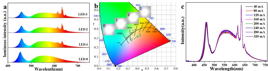
**Fig. 4** (a) Normalized luminous spectra and (b) CIE1931 chromaticity coordinates of devices operated at 320 mA. (c) Normalized luminous spectra of LED-2 operated at different drive currents (40–320 mA).
