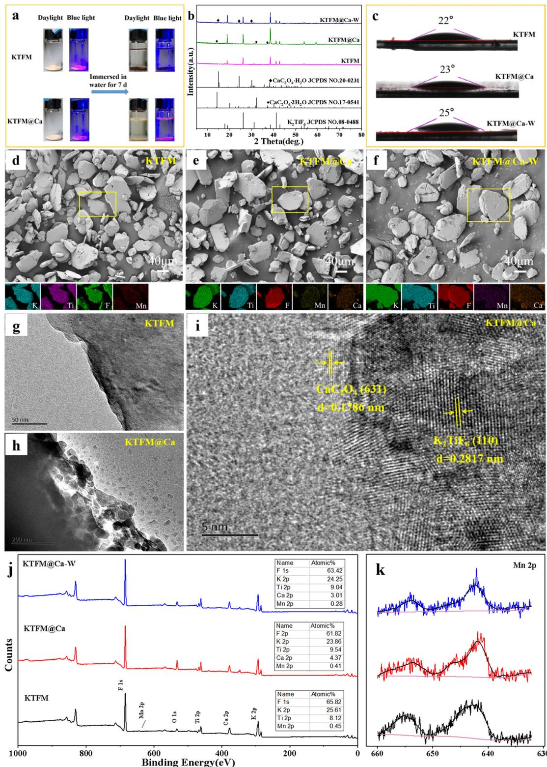
**Fig. 1** (a) Photographs of KTFM and KTFM@Ca samples in air and water. (b) XRD patterns, (c) contact angles, (d)–(f) SEM and EDS mapping images, (g)–(i) TEM images, and (j) and (k) XPS spectra of KTFM, KTFM@Ca, and KTFM@Ca-W.
