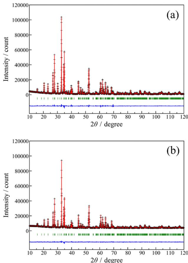
**Fig. 3** Rietveld refinement profiles for the  $\text{Zn}_3\text{Nb}_2\text{O}_8$  (a) and  $(\text{Zn}_{0.80}\text{Co}_{0.20})_3\text{Nb}_2\text{O}_8$  (b) samples. The black cross symbols and the solid red lines represent the observed and calculated intensities, respectively. The difference curves between the observed and calculated patterns are depicted as a blue line at the bottom. The green vertical bars represent the Bragg reflection peak.
