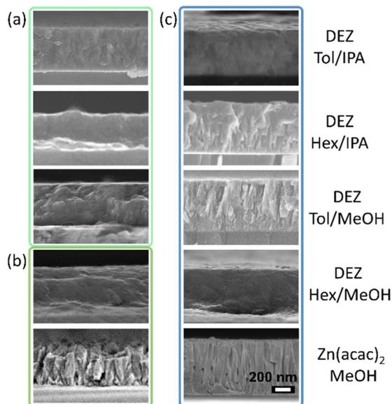
Fig. 4 Cross sectional SEM of ZnO thin films from different precursor solutions at (a) 350 °C, (b) 400 °C and (c) 450 °C, showing that ZnO coatings performed from Zn(acac)<sub>2</sub> exhibited columnar growth and low degree of compactness. In contrast, the use of DEZ and EZI resulted in ZnO film coatings with a high degree of grain coalescence, even at low reaction temperatures. Scale bar applies to all micrographs.
