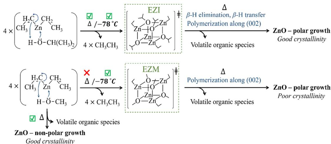
**Scheme 1** Reaction pathways for the formation of ZnO thin film coatings from DEZ and MeOH or IPA precursor solutions using the direct mixture of reagents on the hot substrate (dual-source setup, labelled  $\Delta$ ) or a solution of alkoxide stabilised at low temperature (single-source setup, labelled  $-78\text{ }^{\circ}\text{C}$ ).
