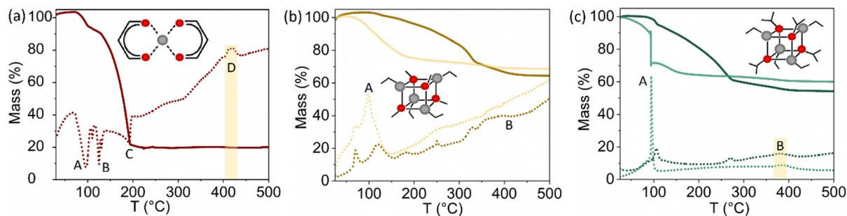
Fig. 1 Thermogravimetric (TGA, full lines) and differential scanning calorimetry (DSC, dotted lines) analyses over the temperature range 25–500 °C of (a)  $\text{Zn}(\text{acac})_2$  in helium or air, (b) EZM in helium (dark) and air (light) and (c) EZI in helium (dark) and air (light). Atoms of Zn are represented with grey spheres and oxygen with red spheres.
