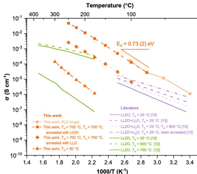
Fig. 5 Arrhenius representation of  $\text{Li}^+$  conductivity of LLZO thin films fabricated in this work compared with literature (undoped LLZO films deposited by PLD).<sup>12,13</sup>
