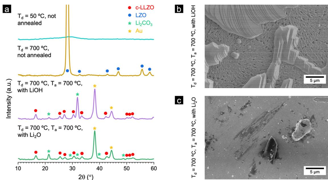
Fig. 3 (a) Grazing-incidence X-ray diffraction patterns of as-deposited (at 50 °C and 700 °C) LLZO films, and Li-garnet films deposited at 700 °C and annealed at 700 °C in presence of Li<sub>2</sub>O or LiOH. Top-view SEM images of LLZO films deposited at 700 °C and annealed at 700 °C with (b) LiOH and (c) Li<sub>2</sub>O.
