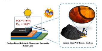
EtOH/H<sub>2</sub>O ratio modulation on carbon for high-V<sub>oc</sub> (1.03 V) printable mesoscopic perovskite solar cells without any passivation
